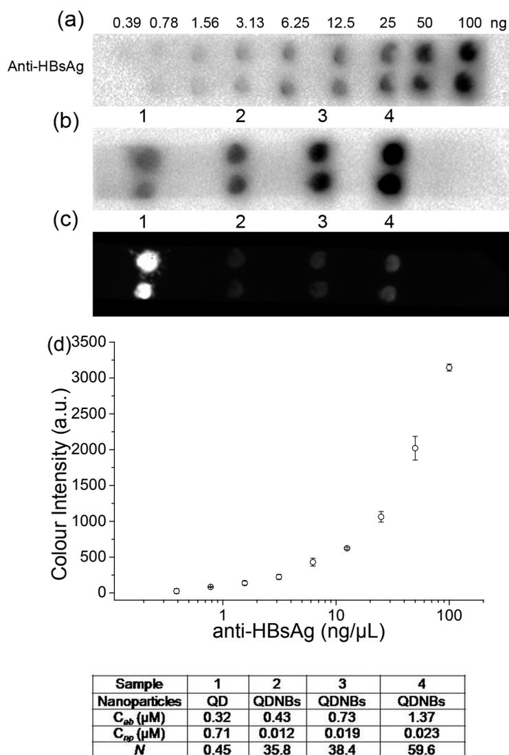
**Figure S4.** Membrane chemifluorescent immunoassay of concentration known anti-HBsAg antibody (a) and antibody conjugates (b), and corresponding fluorescent image (c) of antibody conjugates under UV light illumination. (d) Chemifluorescence intensity of spots against pure antibody concentration.
