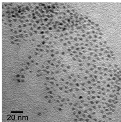
**Figure S3** TEM image of oil soluble CdSe/ZnSe/ZnS QDs (average size:  $5.7 \pm 0.5$  nm).
