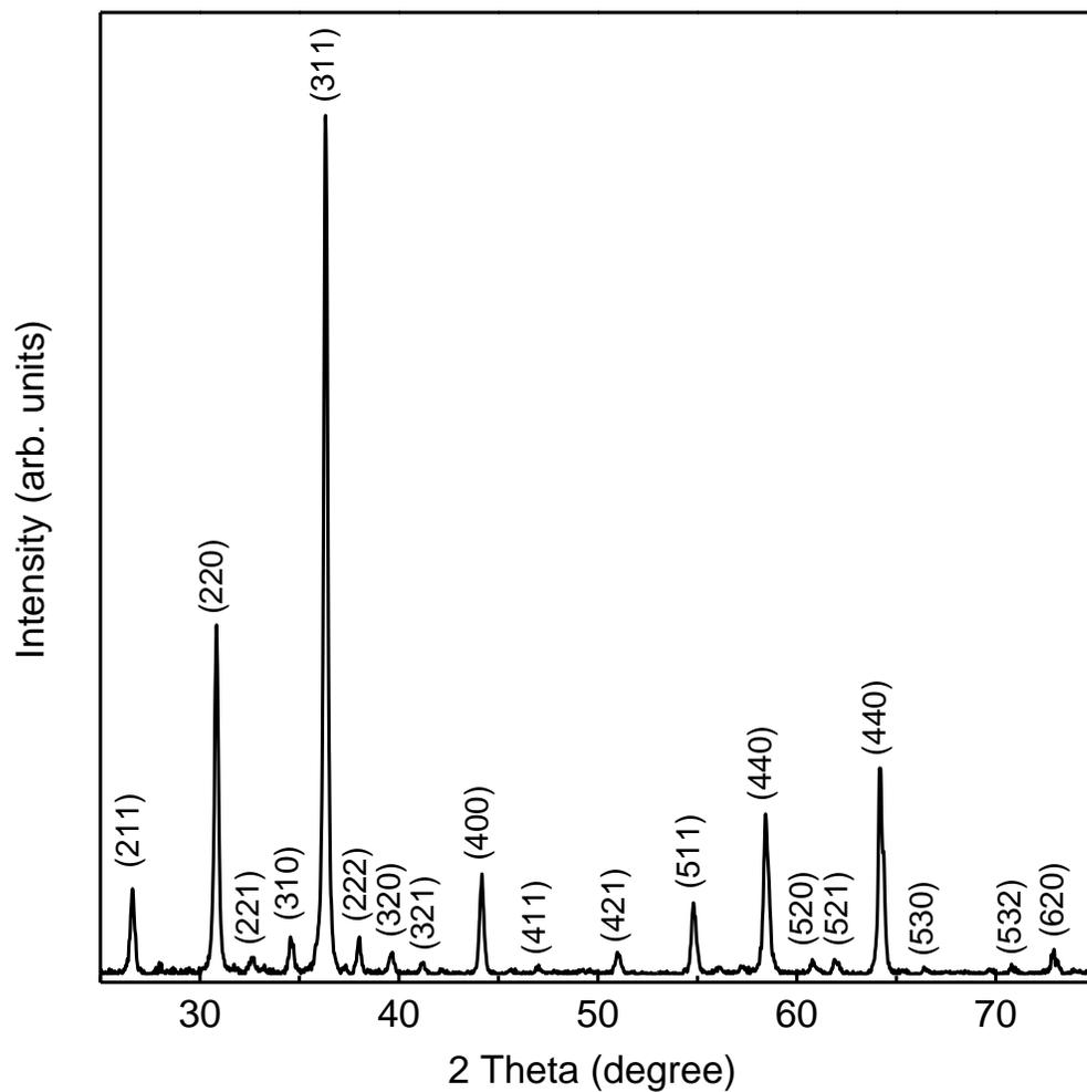
**Figure S1.** XRD pattern of  $\text{LiGa}_5\text{O}_8:\text{Cr}^{3+}$  nanoparticles. The material is identified as cubic  $\text{LiGa}_5\text{O}_8$  (PDF No. 76-199).
