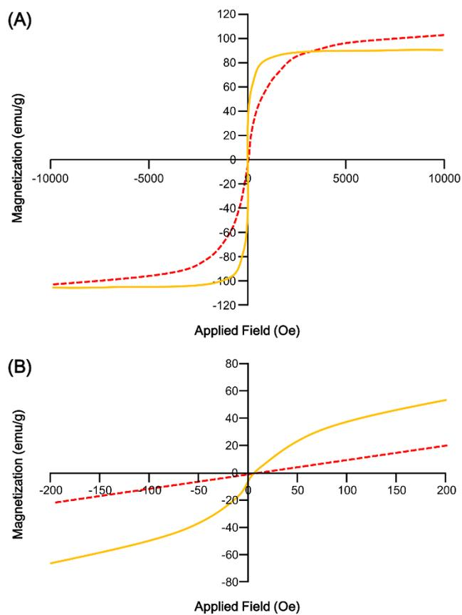
**Fig. S3** (A) The hysteresis loop and magnetic susceptibility of MnMEIO-CyTE777-mPEG NPs (102.8 emu/g) and MnMEIO-CyTE777-(Bis)-mPEG NPs (83.3 emu/g). (B) Coercivity of MnMEIO-CyTE777-mPEG NPs (1.5 Oe) and MnMEIO-CyTE777-(Bis)-mPEG NPs (6.6 Oe).
