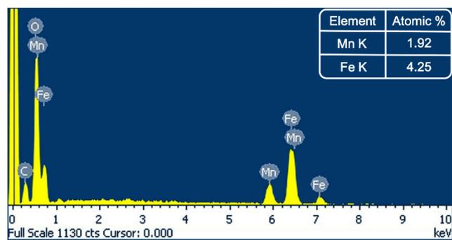
**Fig. S2** EDS spectra of as-synthesized MnMEIO.
