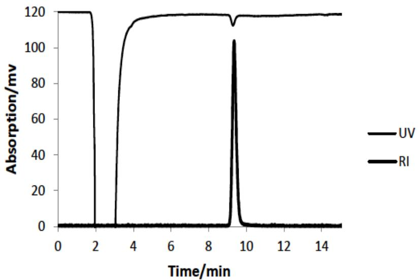
**Figure S3: Analytical and Semi-prep radioHPLC separations
