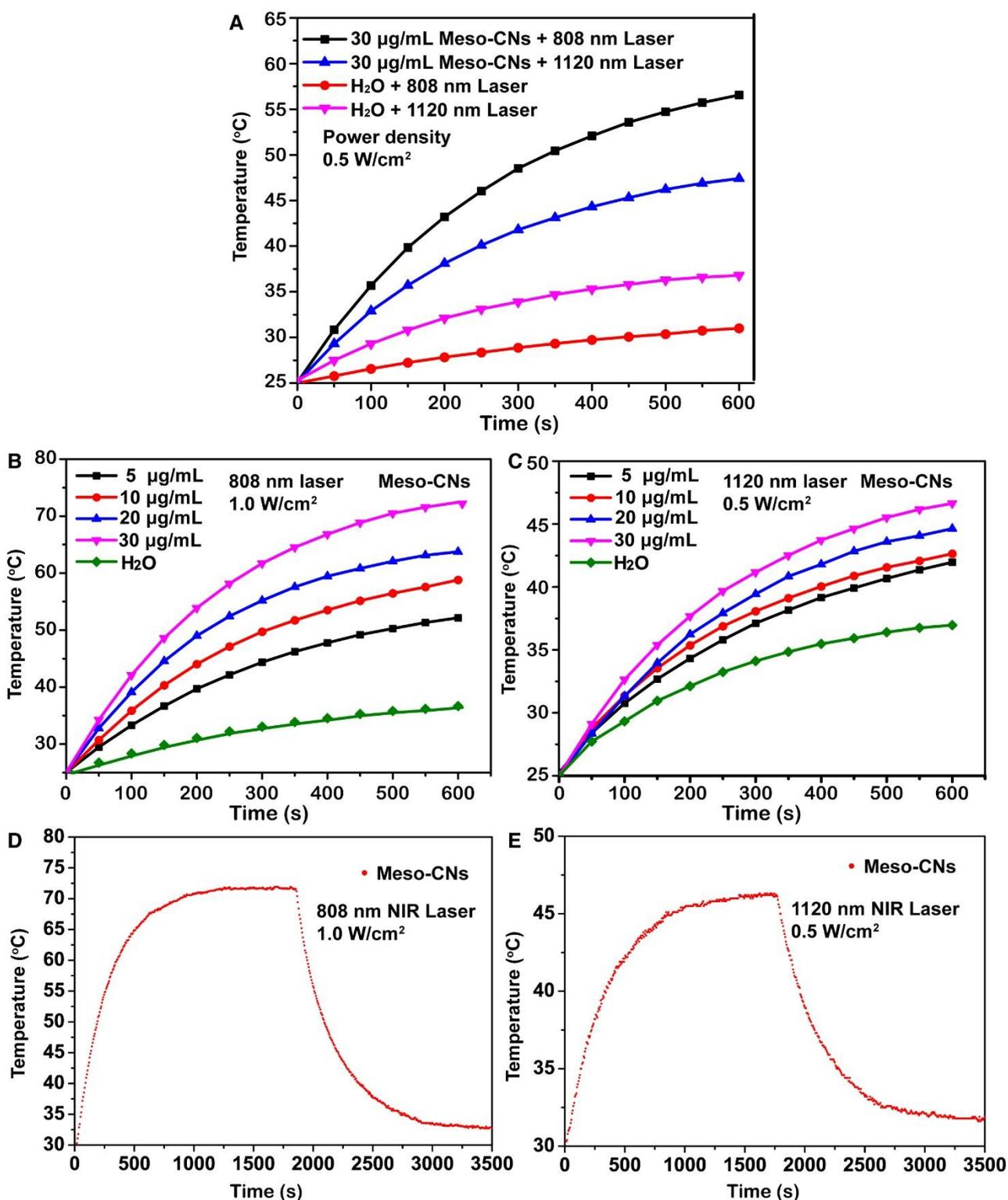
**Figure S4.** (A). Photothermal conversion curves of Meso-CNs and pure water under irradiation with 808 nm or 1120 nm laser (0.5 W/cm<sup>2</sup>). Photothermal conversion curves of pure water and Meso-CNs dispersed in water at different concentrations under irradiation with (B) an 808 nm laser (1.0 W/cm<sup>2</sup>) and (C) a 1120 nm laser (0.5 W/cm<sup>2</sup>). (D). Photothermal response of a Meso-CNs aqueous dispersion
