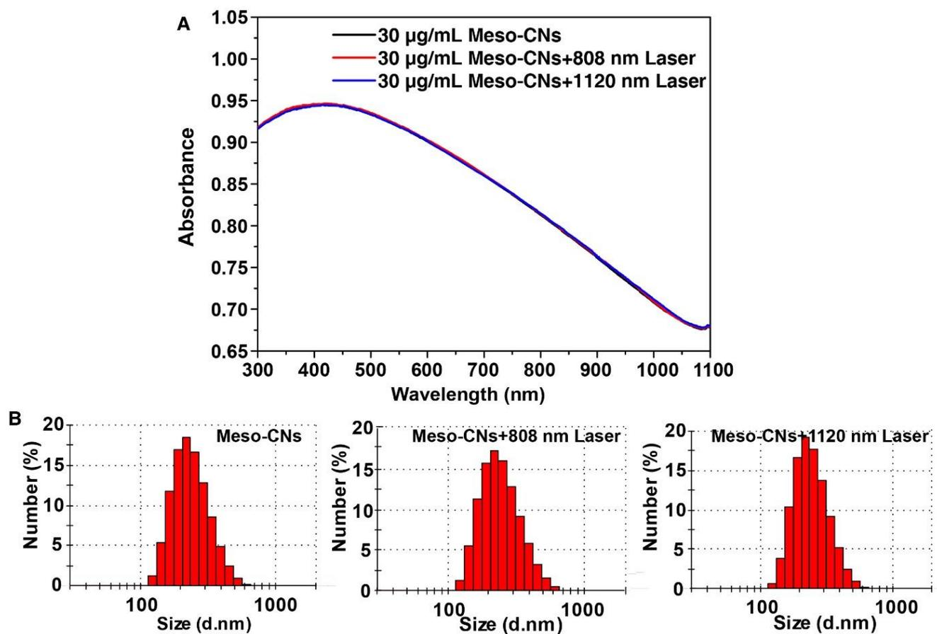
**Figure S5.** **(A)**. Absorption spectra of Meso-CNs in water before and after laser irradiation at 808 nm ( $1.0 \text{ W/cm}^2$ , 30 min) and 1120 nm ( $0.5 \text{ W/cm}^2$ , 30 min). **(B)**. Size distribution of Meso-CNs in water before and after laser irradiation at 808 nm ( $1.0 \text{ W/cm}^2$ , 30 min) and 1120 nm ( $0.5 \text{ W/cm}^2$ , 30 min).
