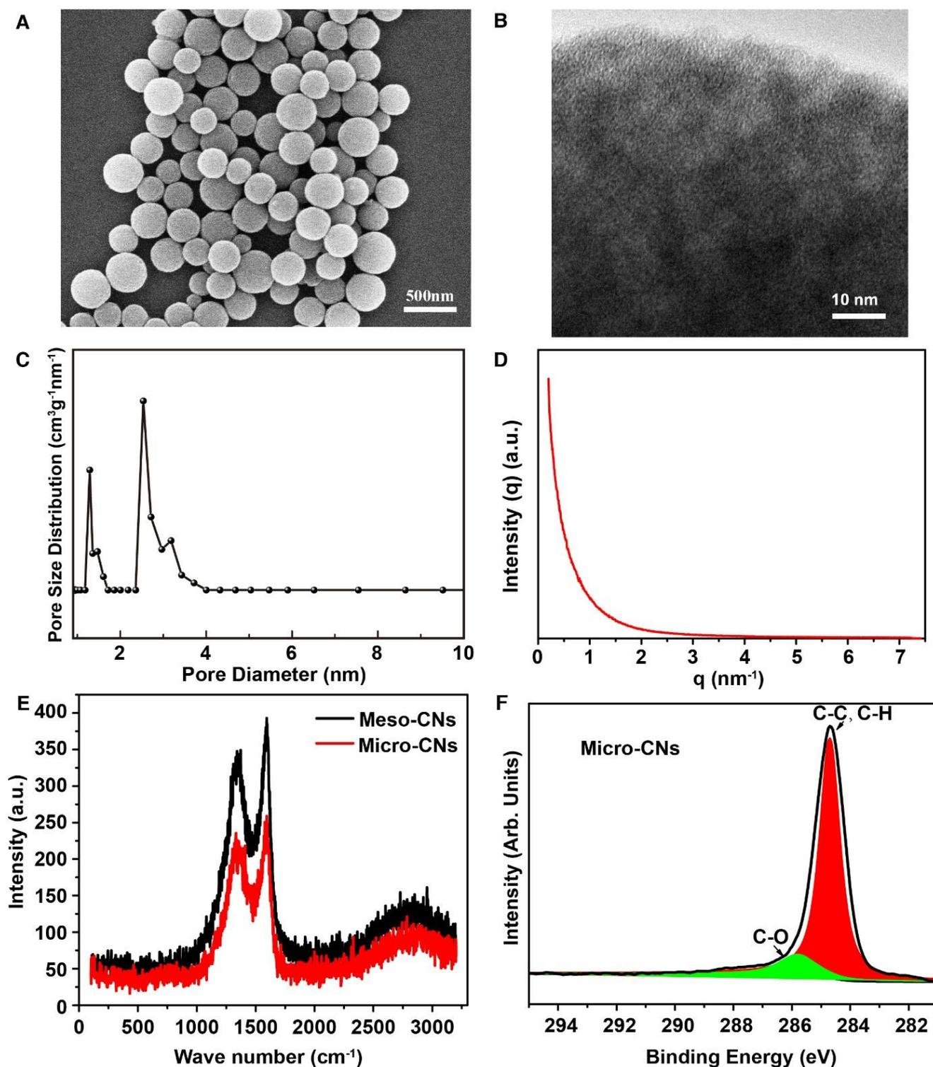
**Figure S1.** (A). A typical SEM image of Meso-CNs. (B). A typical HRTEM image of Meso-CN. (C). Pore size distribution of the Meso-CNs. (D). Small-angle X-ray scattering (SAXS) measurement of the Meso-CNs. (E). Raman spectra of the Meso-CNs and Micro-CNs. (F). XPS patterns of the Micro-CNs.
