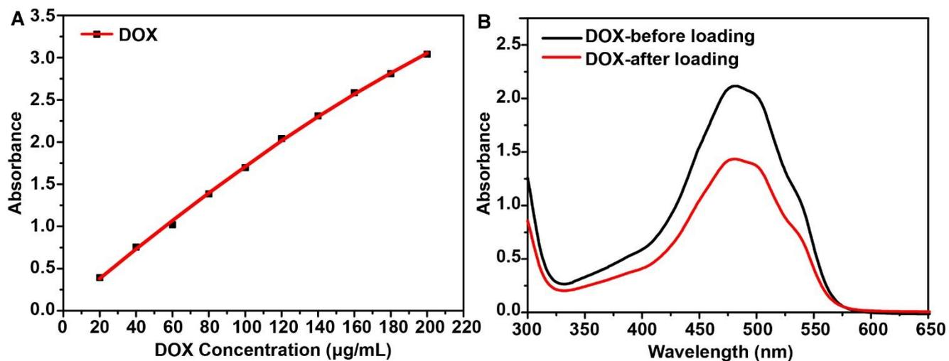
**Figure S6.** (A). Calibration curve for DOX release study. (B). UV-Vis spectra of DOX solution before and after loading in Meso-CNs.
