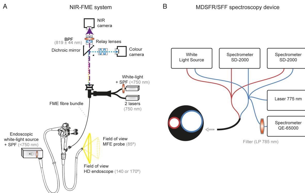
**Figure S1. Schematic representation of the NIR-FME system and the MDSFR/SFF spectroscopy device.**
