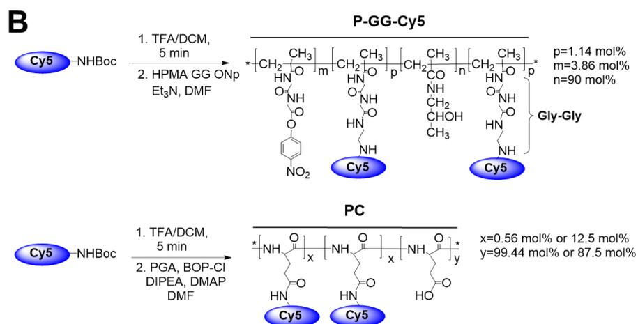
**Scheme S1: Design and synthesis of non-cleavable HPMA copolymer-Gly-Gly-Cy5 (P-GG-Cy5), Always ON PGA-Cy5 (PC) and Never ON PC control probes. (A) Schematic representation of Non-cleavable, Always ON and Never-ON control probes, where no change in fluorescence signal is observed upon incubation with cysteine cathepsins (B) Synthesis scheme of P-GG-Cy5 (upper panel) and PC with 2 different payloads of Cy5 (lower panel) control probes.**
