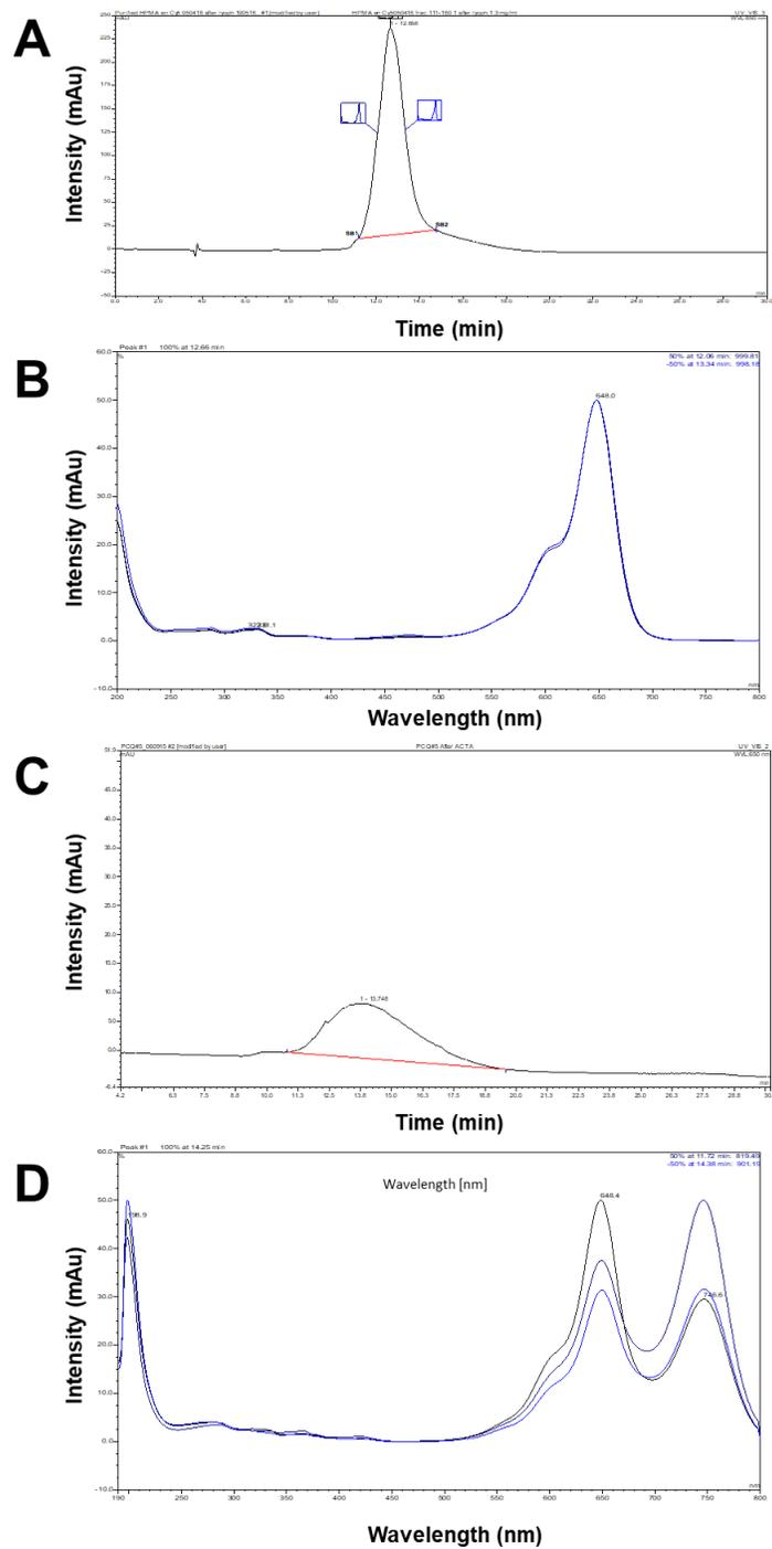
**Figure S3: HPLC characterization of Turn-ON probes.** (A) P-GFLG-Cy5 conjugate chromatogram. (B) Spectrum of the P-GFLG-Cy5 conjugate, with peaks at  $\lambda=600$  and  $650$  nm, indicating Cy5 presence. (C) PGA-Cy5-Quencher (PCQ) conjugate chromatogram. (D) Spectrum of the PCQ conjugate, with peaks at  $\lambda=600$ ,  $650$  and  $750$  nm, indicating Cy5 and quencher presence. 20-100% ACN:DDW with 0.01% TFA, flow rate: 1 mL/min.
