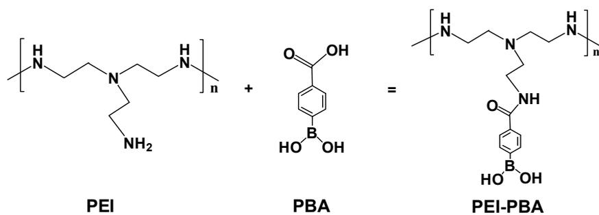
**Figure S1.** Synthesis procedure of PEI-PBA.
