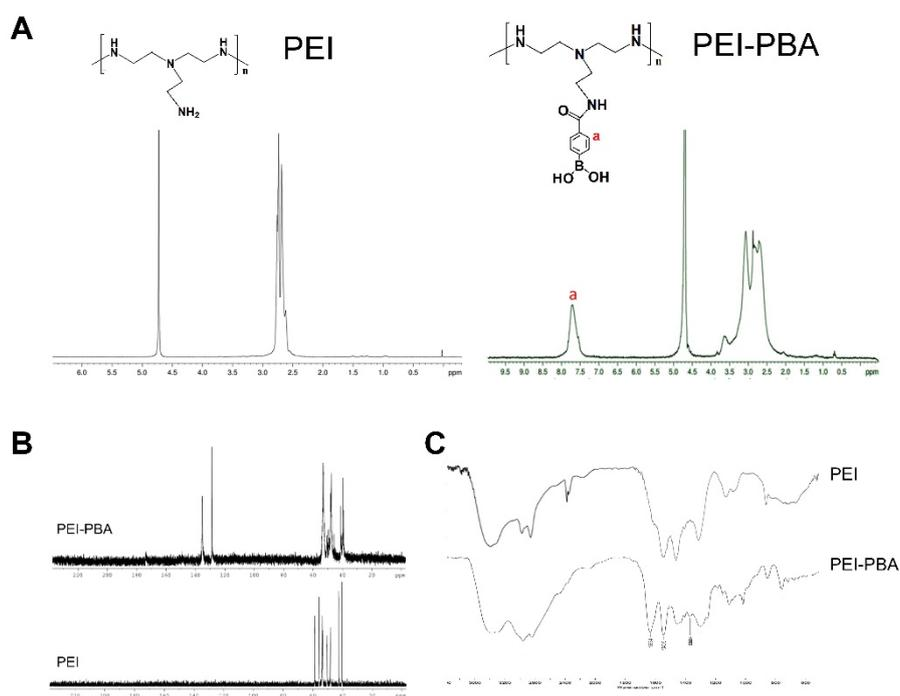
**Figure S2.** Characterization of PEI-PBA. **(A)** The  $^1\text{H}$  NMR spectra **(B)**  $^{13}\text{C}$ -NMR spectra and **(C)** the FTIR spectrum of PEI and PEI-PBA.
