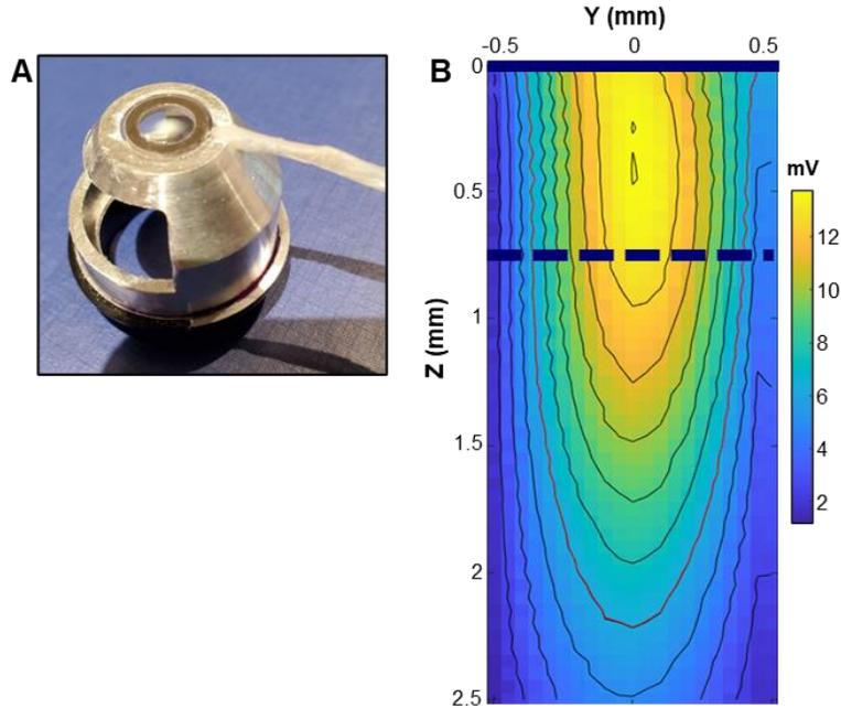
**Figure S1. Overview of the sonication apparatus.** (A) The custom objective lens–ring transducer coupler. (B) Pressure field generated by the ring transducer. The thick dashed line indicates the approximate position of the CAM surface.
