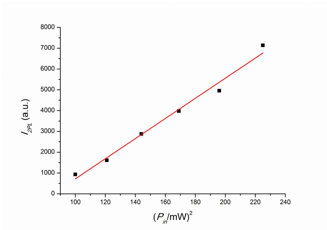
**Figure S4.** Square dependence of 2PL from 760GNRs on the excitation intensity of the 760 nm fs laser.
