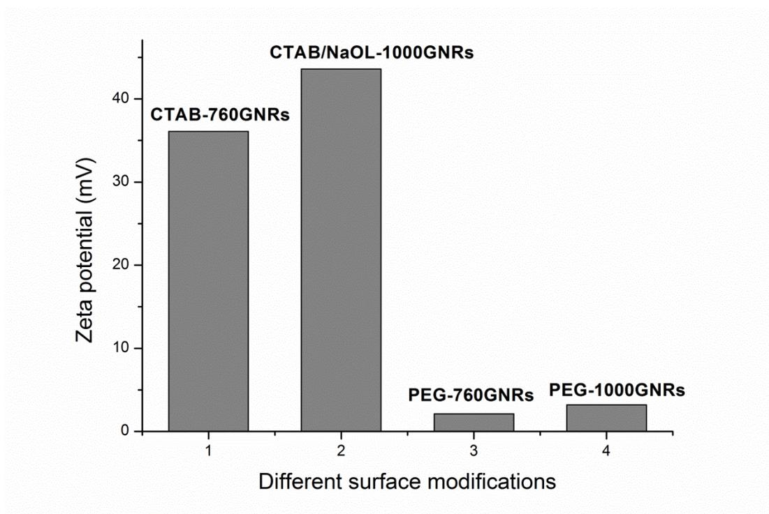
**Figure S2.** Zeta potentials of GNRs with different surface modifications. CTAB-GNRs and CTAB/NaOL-GNRs showed positive charge. After the PEG modification, their zeta-potentials were nearly neutral, which confirmed successful displacement of CTAB/NaOL molecules by PEG polymer.
