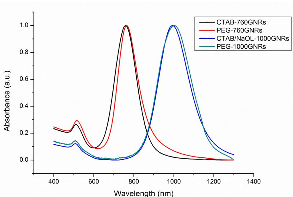
**Figure S1.** UV-Vis-NIR absorption spectra of GNRs before and after PEG modification.
