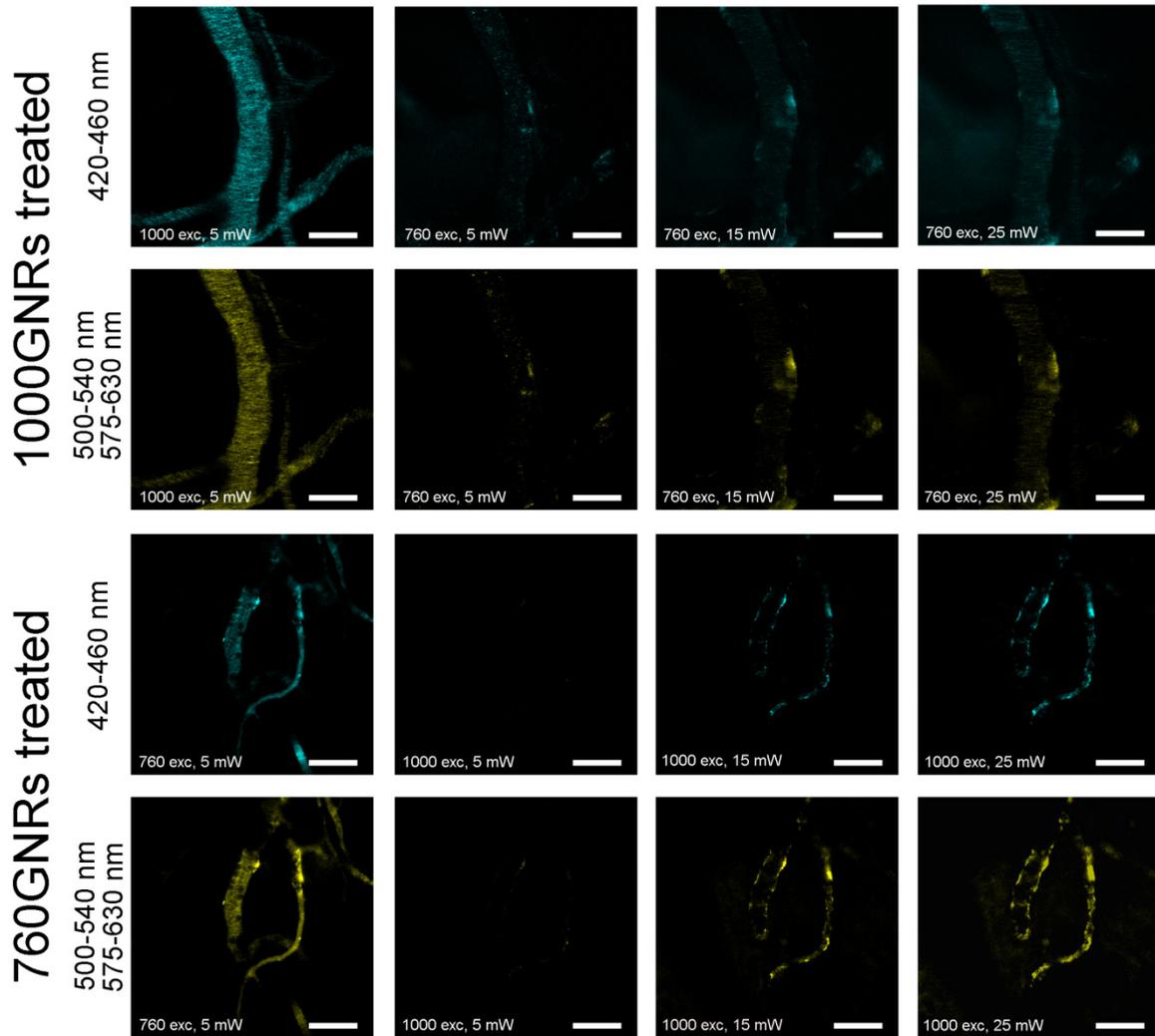
**Figure S10.** Intravital MPL imaging of PEG-1000GNR-stained and PEG-760GNRs-stained mice ear blood vessels, excited by 1000 nm or 760 nm fs lasers. Bright MPL of GNRs in mice ear blood vessels *in vivo* can be excited by a fs laser at a low power when its wavelength is coupled with the longitudinal LSPR band of the GNRs. However, higher power is required to excite MPL of the GNRs when fs excitation wavelength is far away from their absorbance band. Scale bars: 100  $\mu$ m.
