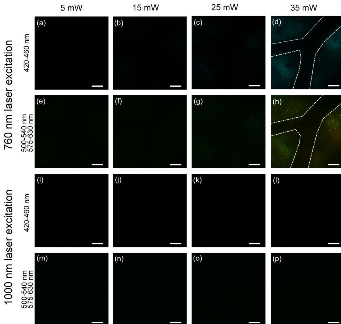
**Figure S11.** Intravital MPL images of brain blood vessels of mice, which were treated with saline. The dotted lines in (d) and (h) indicate the contour of blood vessels and the same areas were excited by 760 nm and 1000 nm fs lasers with different powers. The autofluorescence from brain blood vessels was hardly observed even when the fs excitation power was very high (35 mW), and only autofluorescence from tissue nearby the vessels could be observed. Scale bars: 100  $\mu\text{m}$ .
