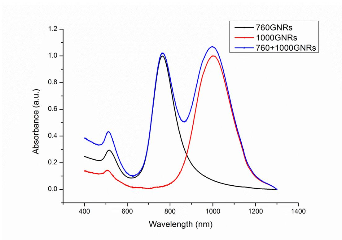
**Figure S9.** Normalized absorption spectra of PEG-1000GNRs, PEG-760GNRs and their mixture.
