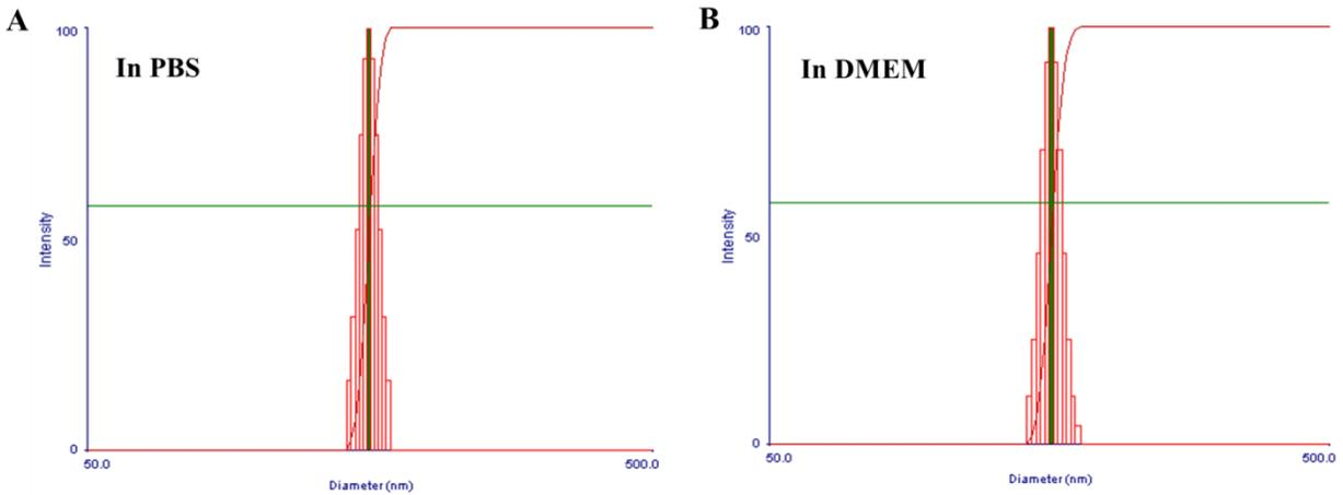
**Figure S2.** DLS measurement of LMMNA in PBS and DMEM showing mean hydrodynamic diameter of (A) ~157 nm in PBS and (B) ~159 nm in 10% FBS supplemented DMEM, respectively.
