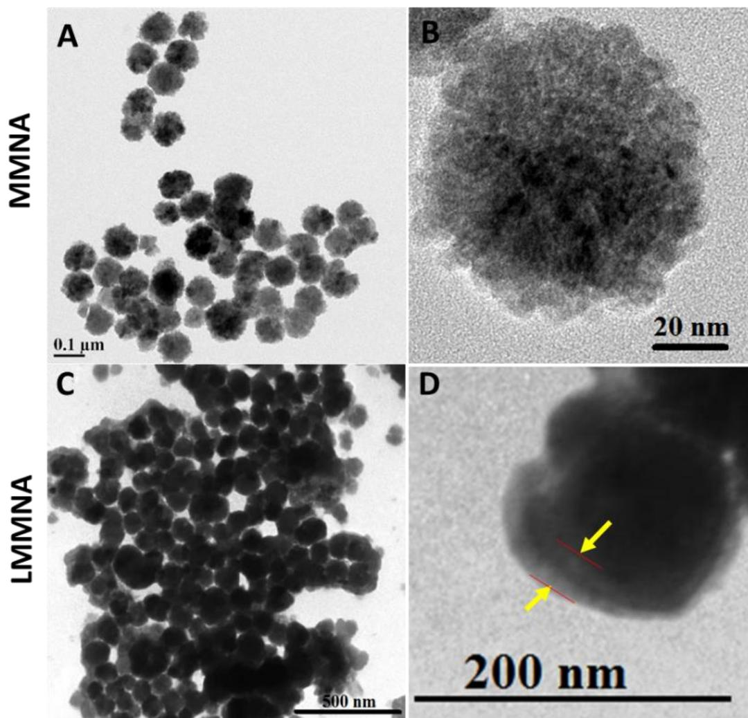
**Figure S1.** TEM images of (A) MMNA, (B) Magnified image of single MMNA, (C) Lipid coated MMNA (LMMNA) and (D) Magnified image of single LMMNA and red lines with yellow arrow marked for thin lipid layer on the surface of MMNA.
