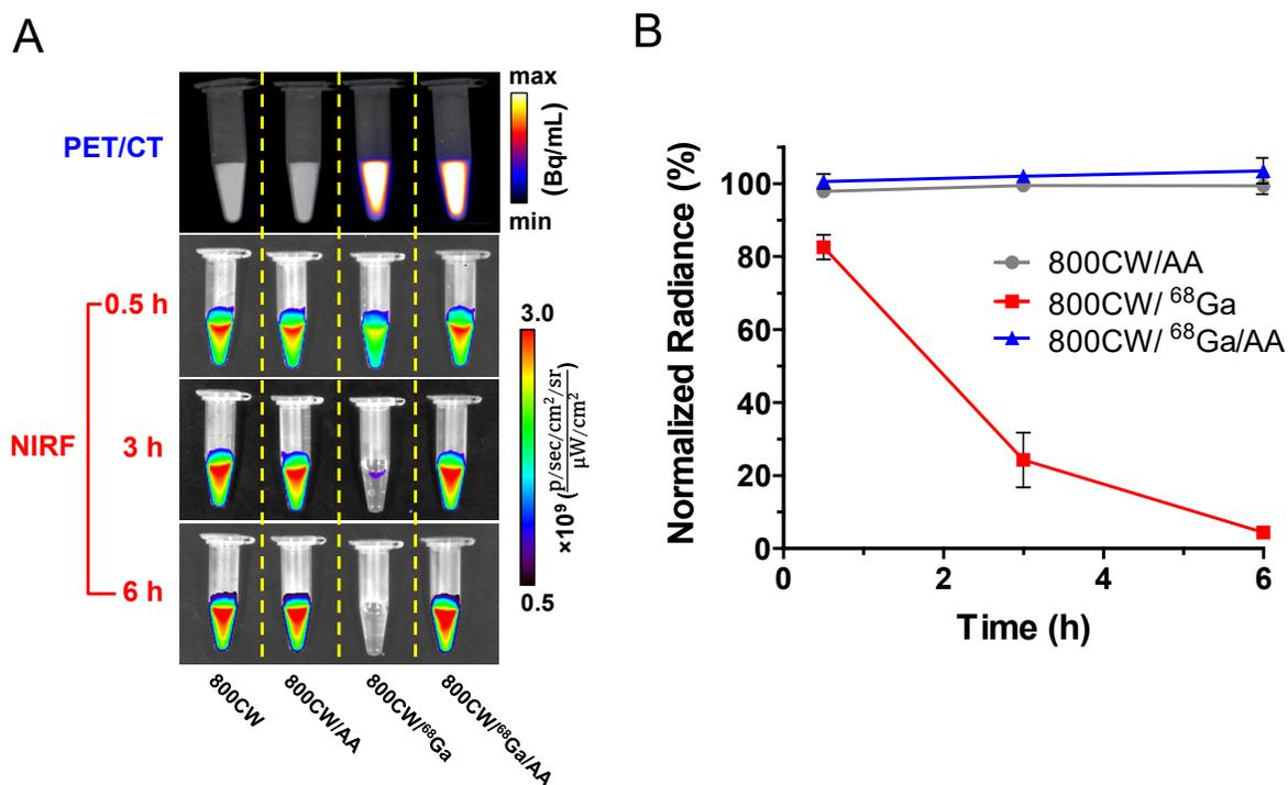
**Figure S4** Fluorescent imaging of irradiated 800CW solutions. **A)** PET/CT and NIRF images reveal that 800CW solution incubated with 20 MBq of <sup>68</sup>Ga experienced a marked radiobleaching. 800CW fluorescence was conserved in solution containing 0.1 (%w/v) AA. **B)** Quantitative ROI analysis of NIRF images shows a drastic decline in normalized radiance of <sup>68</sup>Ga-irradiated 800CW solutions, effect that was counteracted by the addition of AA.
