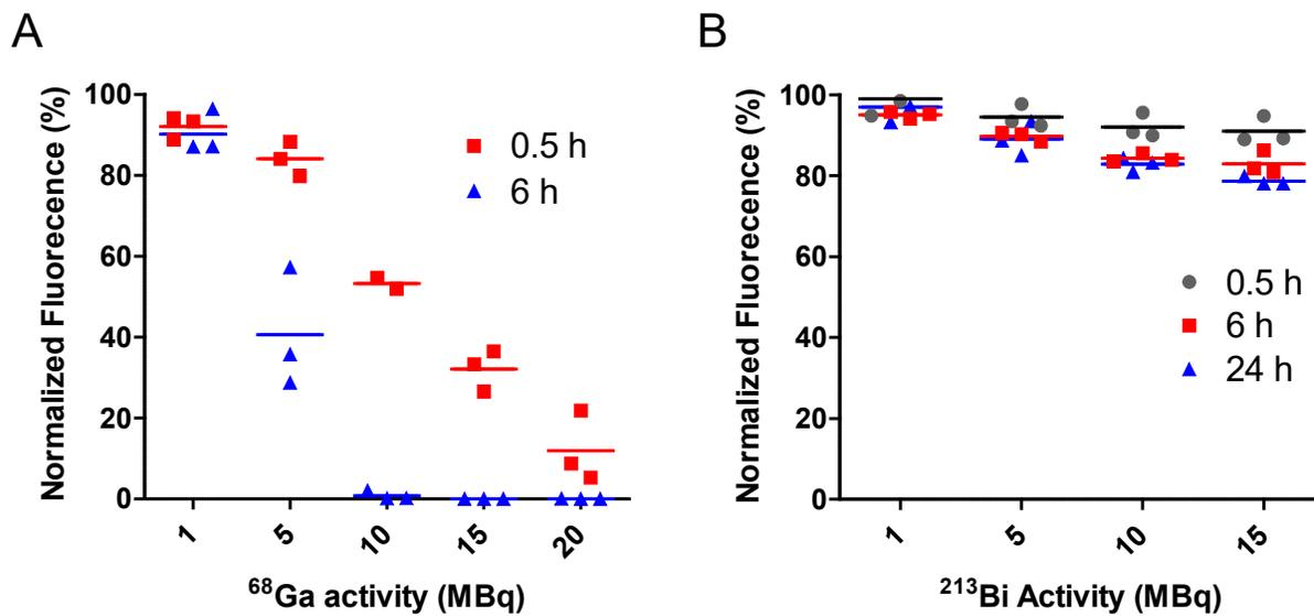
**Figure S3** Time and activity-dependent radiobleaching of irradiated IRDye800CW solutions. Normalized 800CW fluorescence 0.5, 6, and 24 h after exposure to increasing activities of  $^{68}\text{Ga}$  (A) and  $^{213}\text{Bi}$  (B).
