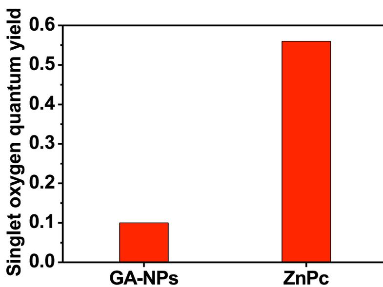
**Figure S5.** Singlet oxygen quantum yield of GA-NPs in aqueous solution using ZnPc in dimethyl formamide as a reference.
