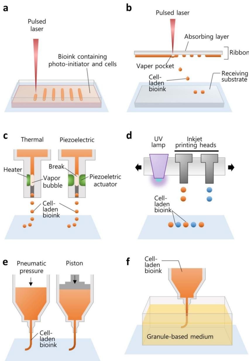
**Figure 1.** Illustrations elucidating the various working principles of 3D printing techniques for building biological constructs. The techniques include (a) SLA, (b) laser-assisted printing, (c) inkjet printing, (d) multi-jet modeling, (e) extrusion printing, and (f) granule-based medium-assisted printing.
