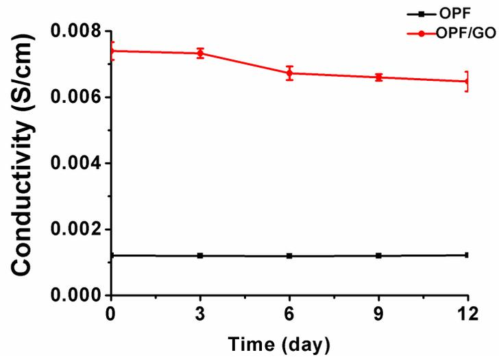
Figure S1. The time-dependent measurement of the electrical conductivity of OPF (black line) and OPF/GO (red line) hydrogel. (n=3/group)
