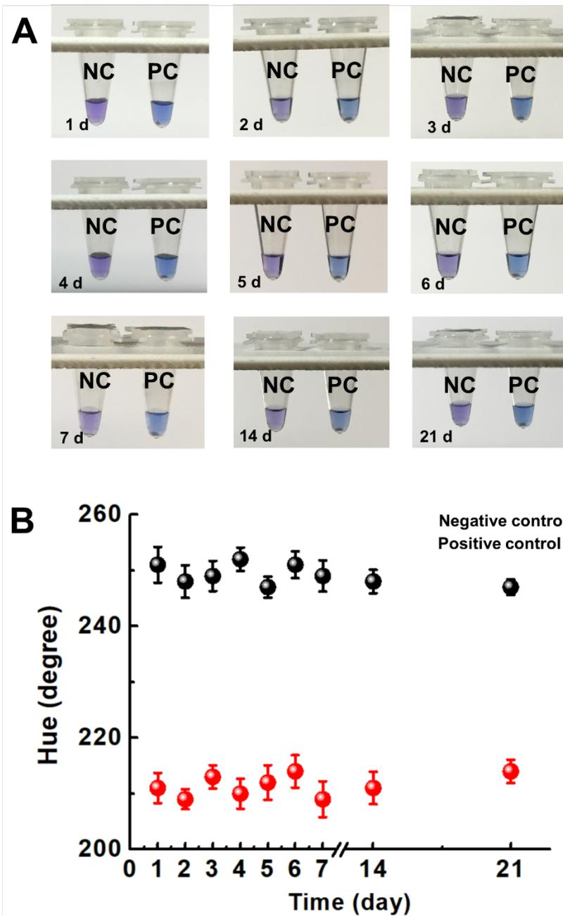
**Figure S8 Stability evaluation of HNB indicator in non-buffered LAMP solution after LAMP reaction.** (A) Serial optical images of LAMP amplification products including negative control (NC) and positive control (PC). (B) Hue value comparison of LAMP amplification products stored at room temperature at different time (days). Error bars denote s.d. (n=3).
