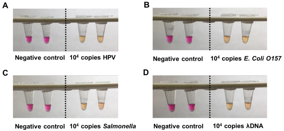
**Figure S5 pH value change of different nucleic acid targets detection in non-buffered LAMP solution after 60-min LAMP reaction. (A) HPV 16, (B) *E. coli* O157, (C) *Salmonella*, and (D)  $\lambda$ DNA. 100  $\mu$ M phenol red was used as the pH indicator.**
