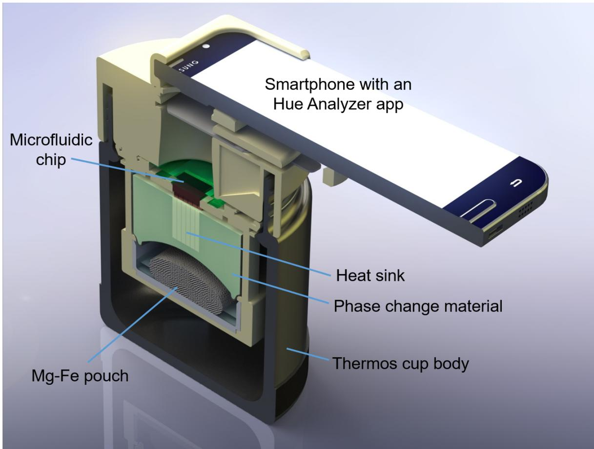
**Figure S3** Cross-section of our smart cup-based POC diagnostic platform for HPV-associated cancer screening.
