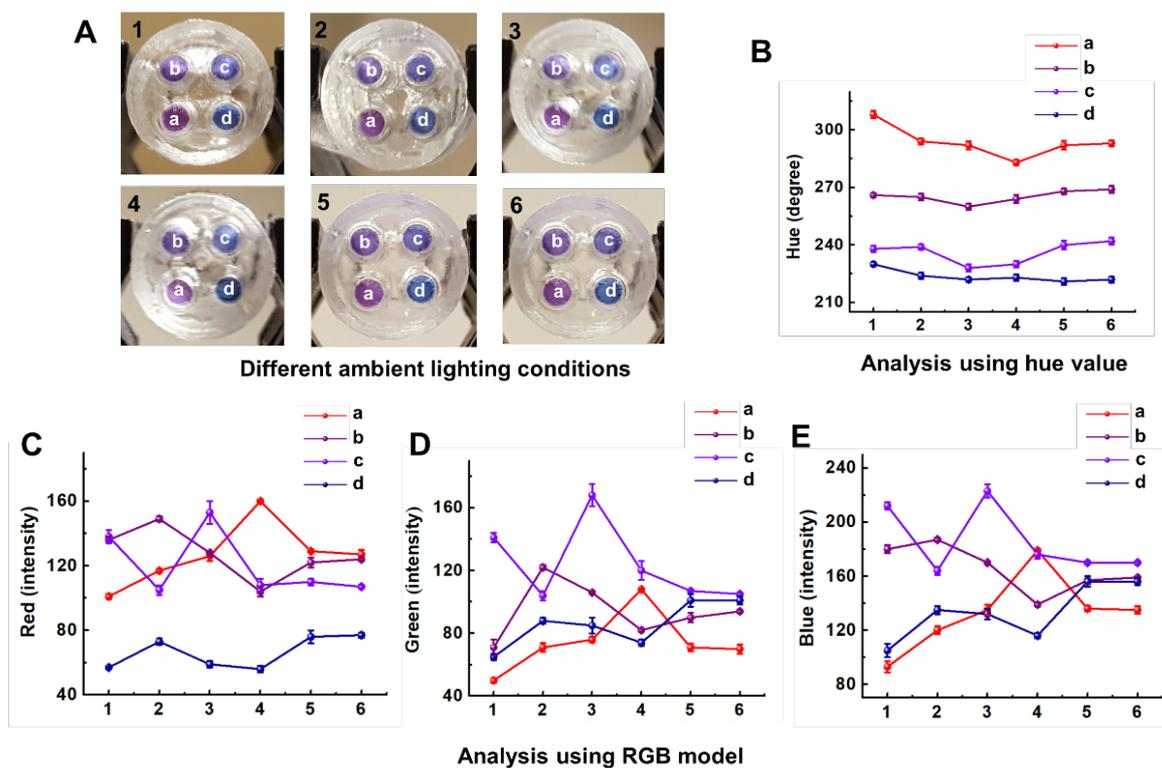
**Figure S7 Reliability comparison of colorimetric detection between hue value analysis and RGB model.** (A) Serial optical images of HNB indicator in the presence of  $Mg^{2+}$  ions (a: 16 mM, b: 12 mM, c: 8 mM, and d: 4 mM) under different ambient lighting conditions. (B) Hue values of HNB in chamber a, b, c and d under different ambient light. (C-E) Red, Green, and Blue values of HNB in chamber a, b, c and d under different ambient light. Error bars denote s.d. ( $n=3$ ).
