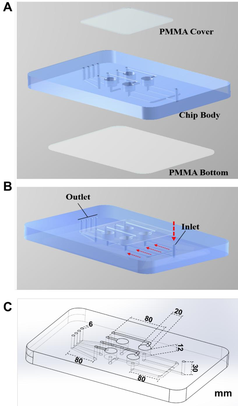
**Figure S2 Schematic illustration of microfluidic chip housing four reaction chambers.** (A) An exploded view of the chip used for detecting multiple HPV genotypes. The chip consists of three layers: one top PMMA film, one PMMA chip body, and one PMMA bottom. The various features of the chip body were milled with a computer numerical control (CNC) machine. (B) Assembled microfluidic chip. (C) CAD illustration of the chip.
