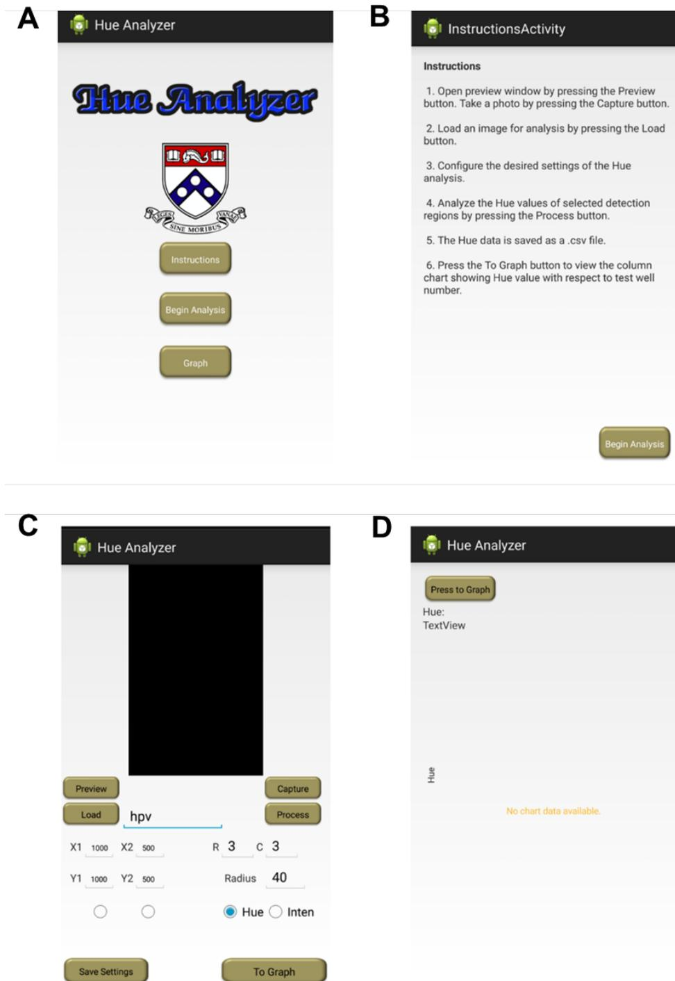
**Figure S1 Screenshots of the interfaces of our custom Hue Analyzer app for hue value quantification and HPV-associated cancer screening. (A) Main menu, (B) Instructions, (C) Parameter settings and image capturing, and (D) Data analysis and result reporting.**
