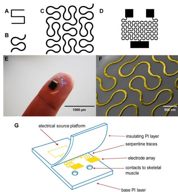
**Figure 1.** (A) A basic element of a fractal pattern. (B) The hard edges were replaced by arcs for contour. (C) Peano curve variation shown to provide hard-metal traces with tensile strength. (D) The electrode array Peano curve. (E) The flexible microelectrode array (MEA), including a source platform that is 1 cm by 1 cm in size. (F) Scanning electron microscope image of the gold Peano curve electrode. (G) Schematic of the device components.
