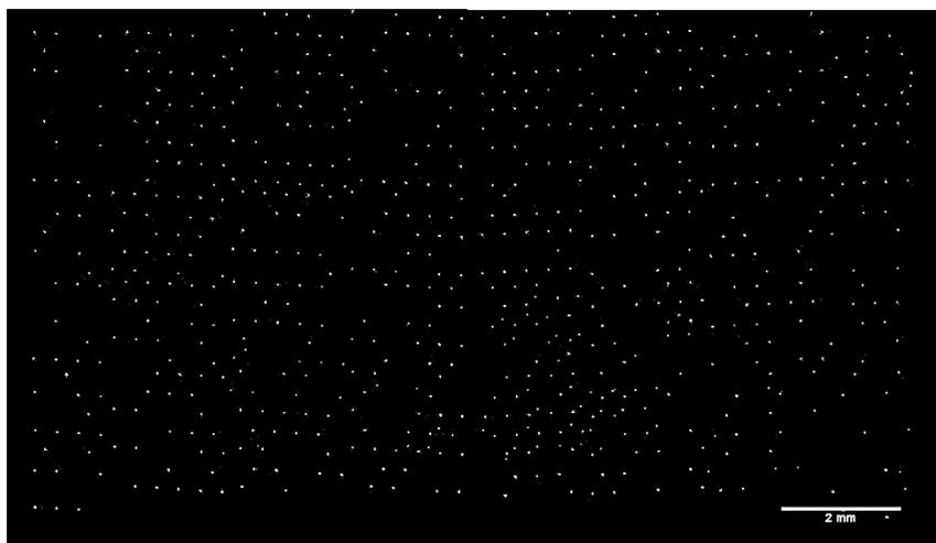
E. Fluorescent samples caught in the hydrodynamic traps at 30  $\mu\text{L}/\text{min}$  flow rate
