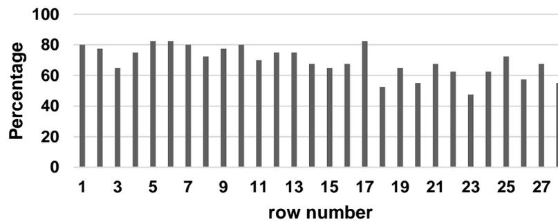
Percentage of traps occupied for 10  $\mu\text{L}/\text{min}$  flow rate
