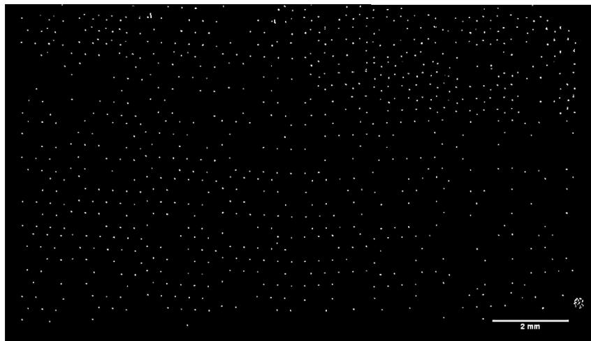
D. Fluorescent samples caught in the hydrodynamic traps at 20  $\mu\text{L}/\text{min}$  flow rate
