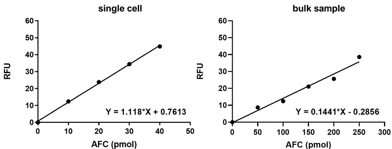
**Figure S4.** Standard curves were taken using the microfluidic device (left) for single cell measurement and a 96-well plate (right) for bulk sample measurement. Different amounts of AFC standard were placed in the microfluidic platform as well as in the well-plate following the assay kit protocol. The fluorescence coming from each of the sampled micro chamber and each well of the 96-well plate was measured. This was used for the interpolation of the GrB activity in the assay experiment.
