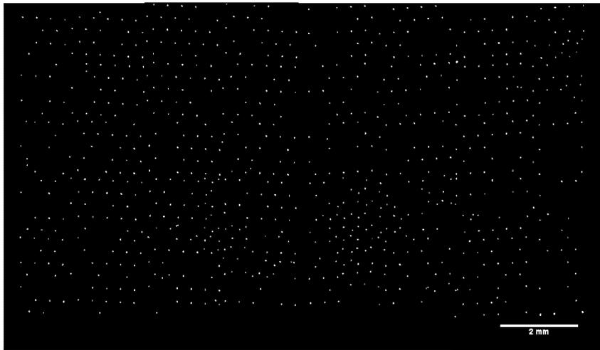
C. Fluorescent samples caught in the hydrodynamic traps at 15  $\mu\text{L}/\text{min}$  flow rate
