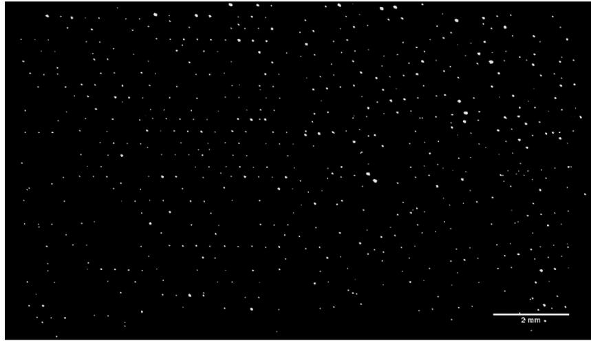
A. Fluorescent samples caught in the hydrodynamic traps at 5  $\mu\text{L}/\text{min}$  flow rate
