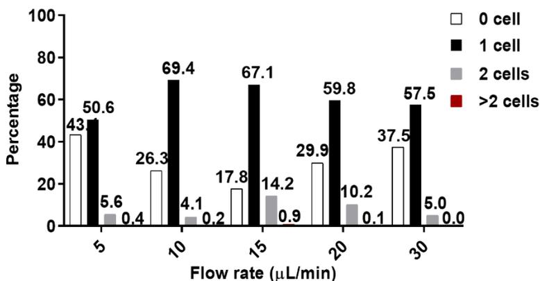
F. Percentage of trap occupancy at different flow rates. The percentage of traps with single capture is shown by the black solid bar, double capture by gray solid bar, while more than 2 cells captured is shown by red bar
