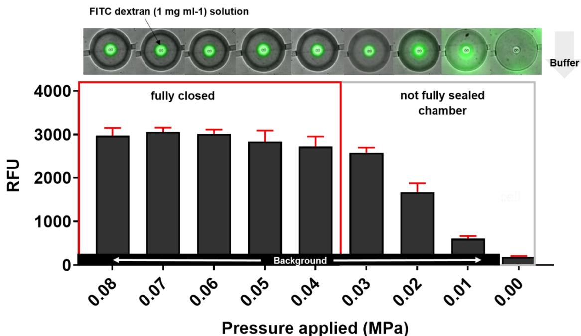
**Figure S3.** To create a sealed microchamber, the pneumatic valves were applied with positive pressure using an air pump (ULVAC DA-60S). The working pressure was determined by actuating the valves at different pressure and measuring the fluorescence of the compartmentalized FITC dextran solution (1 mg ml<sup>-1</sup>, Sigma-Aldrich) inside and outside of the chamber. An applied pressure of 0.07 MPa was later on used in the conduct of the GrB activity assay experiment.
