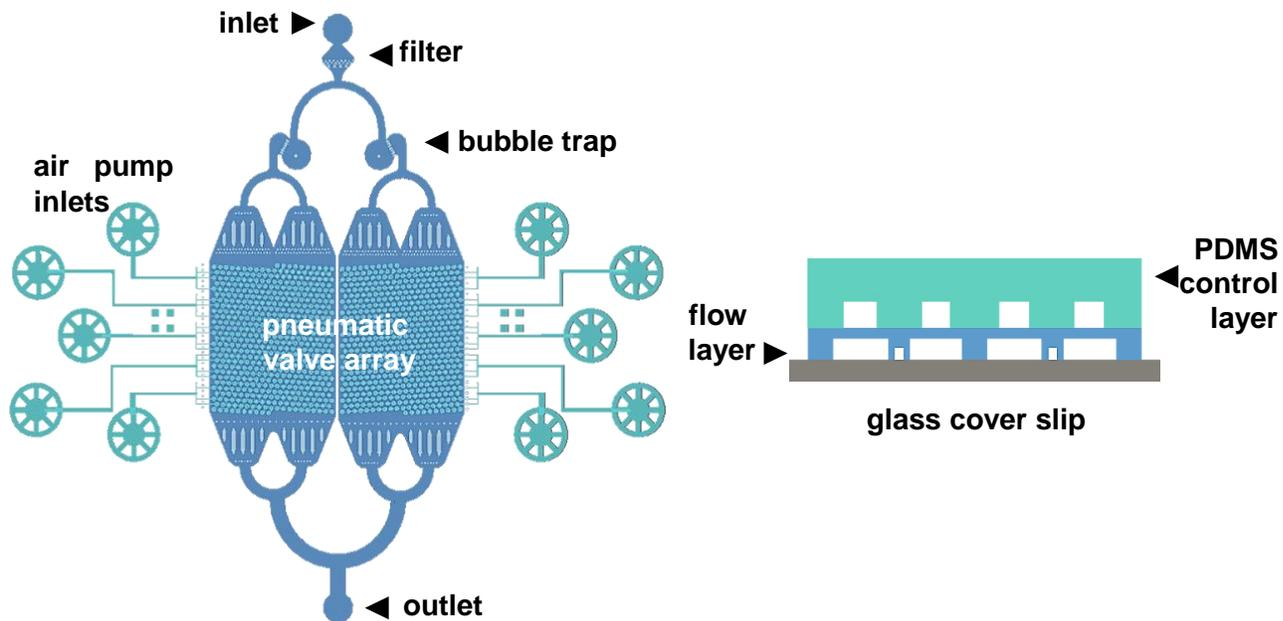
Left, combined CAD design of the control (cyan) and flow layer (blue) moulds.
