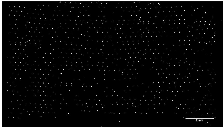
B. Fluorescent samples caught in the hydrodynamic traps at 10  $\mu\text{L}/\text{min}$  flow rate
