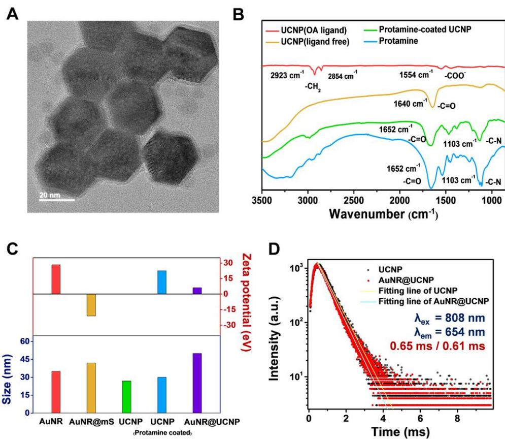
**Figure S3.** Protamine-coated UCNP with (A) TEM images and (B) FTIR spectrum. (C) Zeta potential and hydrodynamic diameter of each nanomaterial. (D) Lifetime measurement of UCNP and AuNR@UCNP.
