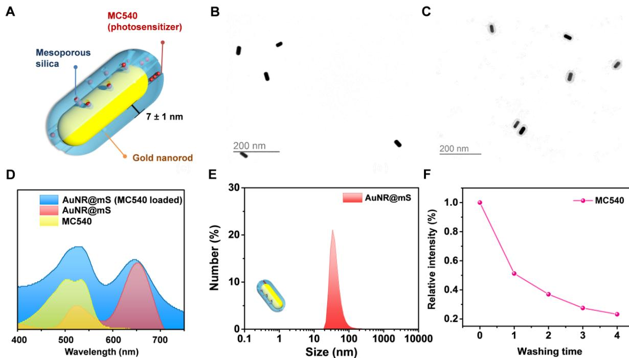
**Figure S1.** (A) Schematic of AuNR@mS (MC540 loaded). TEM images of (B) AuNR and (C) AuNR@mS. (D) Absorbance spectrum of AuNR, MC540, and AuNR@mS-MC. (E) DLS analysis of AuNR@mS-MC. (F) Loading diagram of photosensitizer, MC540 with centrifugations and washed four times to ensure that MC540 was loaded in AuNR@mS.
