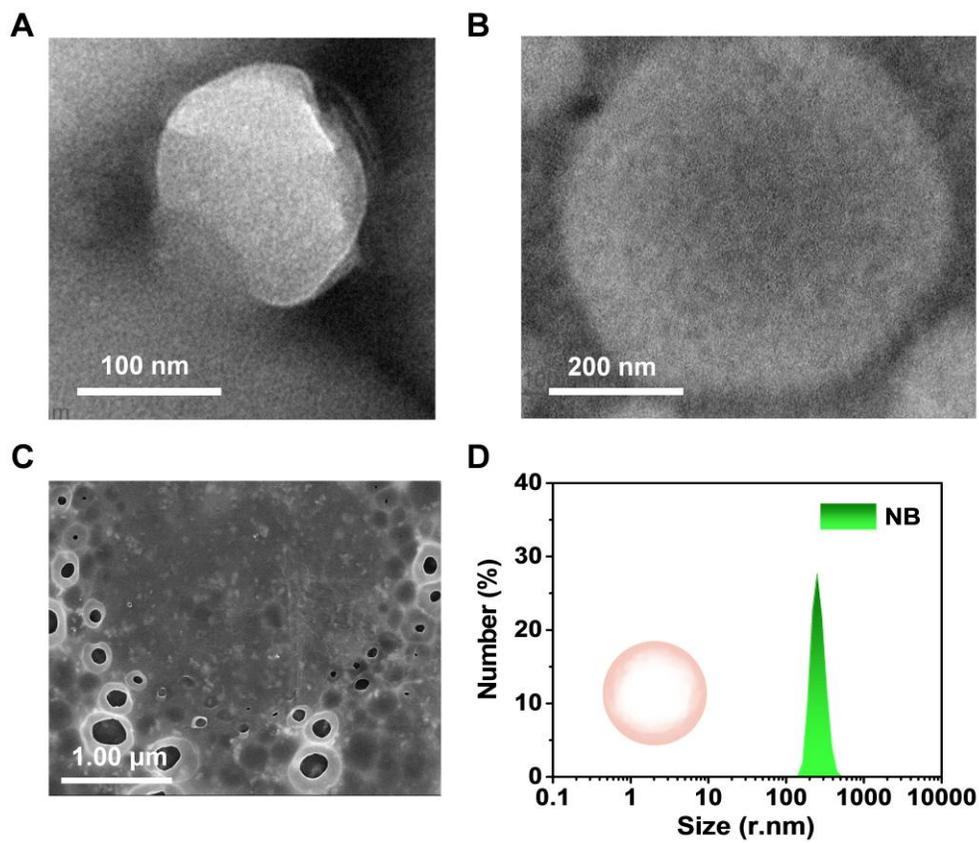
**Figure S4.** TEM images of NB at approximately (A) 100 nm and (B) 200 nm. (C) SEM image and (D) DLS analysis of NB.
