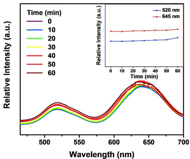
**Figure S5.** The absorption spectrum of AuNR under 808 nm laser irradiation for an hour (monitoring at 520 nm and 645 nm).
