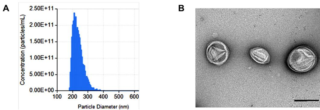
**Figure S6. Characterisation of SN38 liposomes.** (A) Q-nano histogram for liposome concentration and size distribution. (B) Transmission electron microscopy (TEM) image of liposomes with encapsulated SN38. Scale bar denotes 200 nm.
