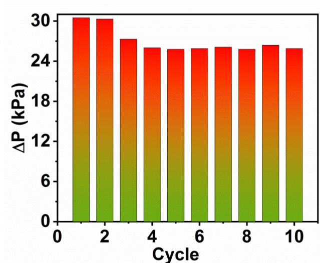
**Figure S5.** Reuse of 6-PAAC-30 (1.0 mg) in 20 mM H<sub>2</sub>O<sub>2</sub> decomposition.
