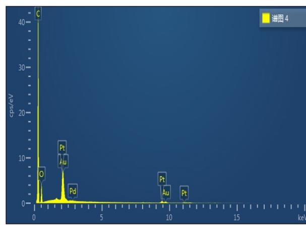
**Figure S2.** EDX spectroscopy analysis of 6-PAAC-30.
