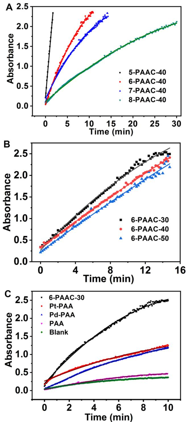
**Figure S4.** Time-dependent absorbance changes of TMB at 652 nm varied with different catalysts used for testifying the POD activity. Experimental conditions: MES-AC buffer solution, pH 4.5; TMB, 0.8 mM; H<sub>2</sub>O<sub>2</sub>, 1.0 mM; catalysts, 1.0 mg; measured at 37 °C.
