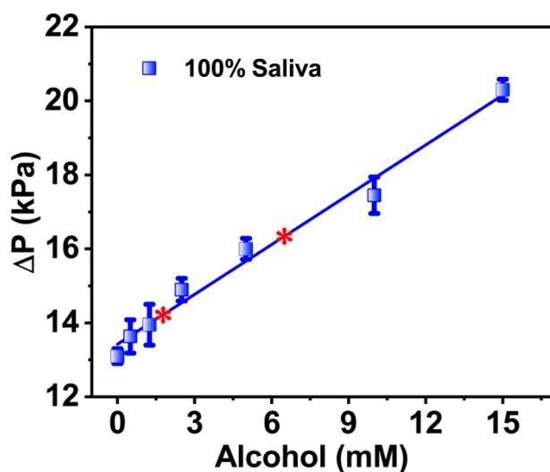
**Figure S6.** The linear correlation between  $\Delta P$  and alcohol concentration in 100% saliva calculated from the curve in 40% saliva sample (blue line of Figure 4A, in manuscript). Red snowflakes represent DUI and DWI, respectively.
