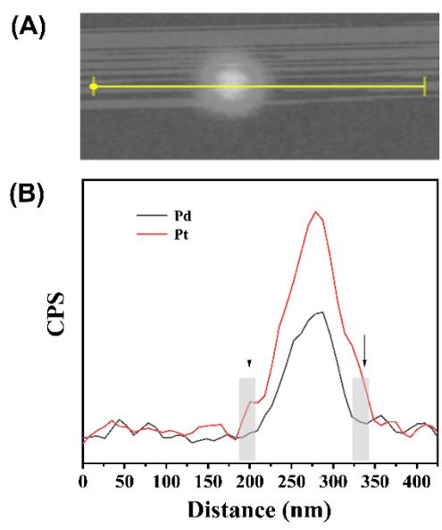
**Figure S1.** (A) The image of target nanoparticle and scan path. (B) EDS line scans of Pd and Pt recorded from a Pd@Pt core-shell nanoparticle. The two regions in gray indicate the ~20 nm thickness of the Pt shell.
