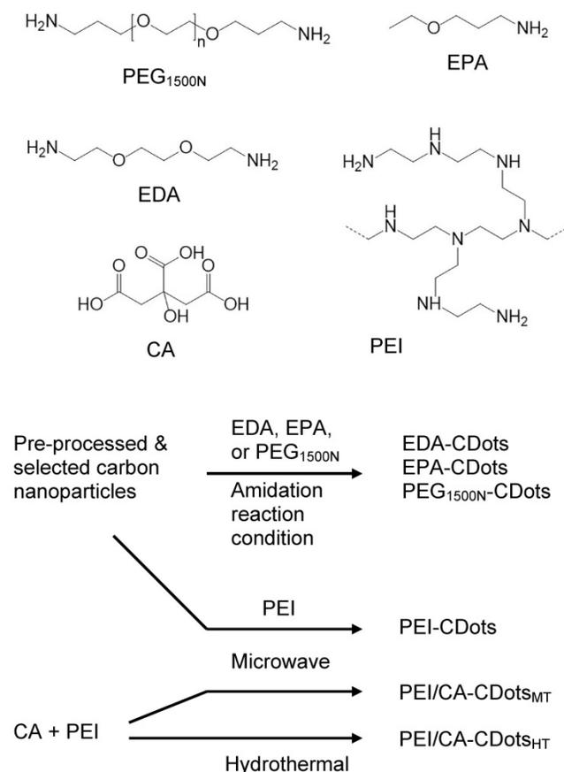
**Figure 5.** Selected organic molecules used for surface functionalization and/or as precursors for the various CDots, and the different reaction schemes for syntheses of the CDots under different processing conditions, including the chemical functionalization (amidation) and thermally induced functionalization
