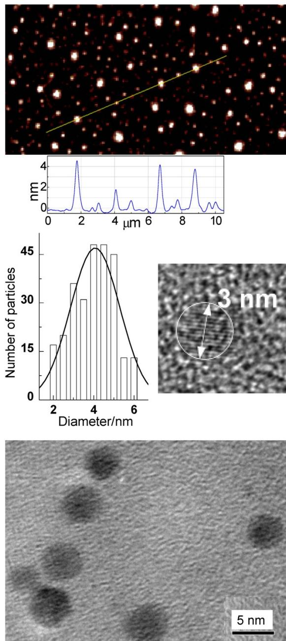
**Figure 4.** Top: Atomic force microscopy (AFM) imaging results for EDA-CDots on mica substrate, with height profiles of some dots along the line highlighted; Middle: (left) The size distribution based on height analyses of multiple AFM images, fitted with the Gaussian distribution curve, and (right) a high-resolution transmission electron microscopy (TEM) image illustrating the carbon core in a dot; Bottom: TEM images of the EDA-CDots. (Reprinted with permission from ref. [19])
