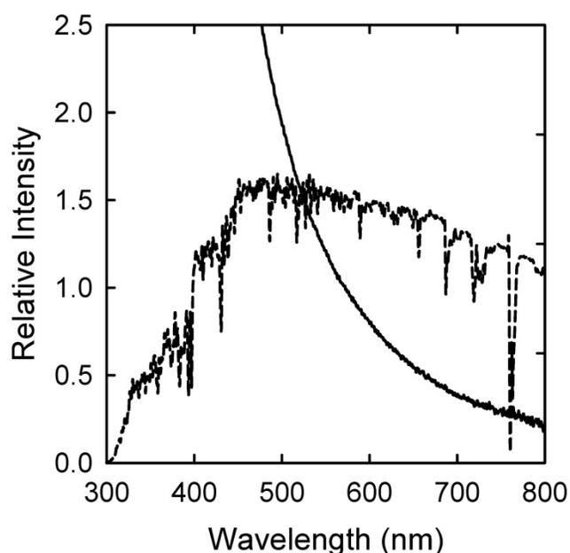
**Figure 2.** The observed absorption spectrum of broadly distributed CDots in aqueous solution (solid line), which is essentially the same as that of the aqueous dispersed carbon nanoparticles used for the CDots, except for less scattering effects, and the comparison with the solar spectrum at the sea level (dashed line). (Reprinted with permission from ref. [39])
