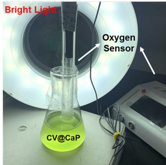
**Fig. S3.** Photograph of the oxygen sensor device testing the oxygen productions in the CV@CaP sample under the bright light.
