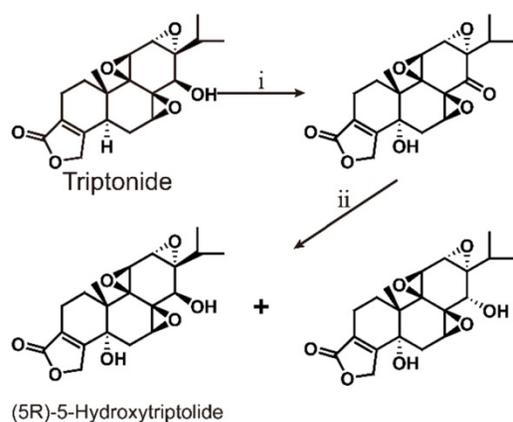
**Scheme 6.** Total synthesis of (5R)-5-Hydroxytriptolide. i)  $\text{SeO}_2$ , heat reflux 10 h; ii)  $\text{NaBH}_4$ , 2 h
