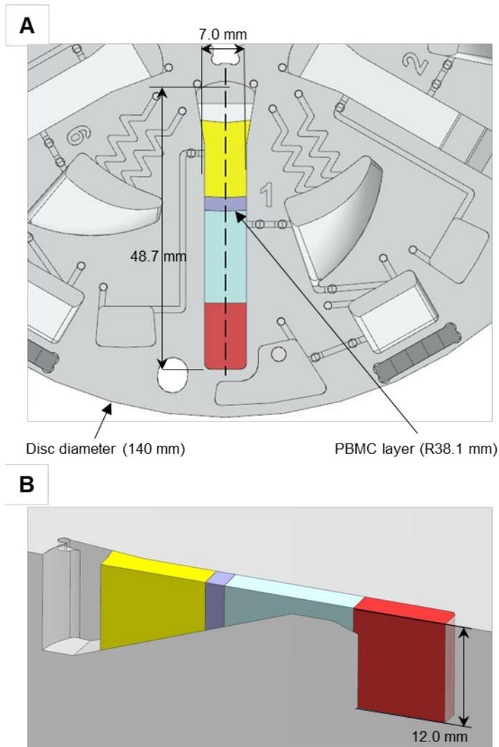
**Figure S5. Dimension of CTCD.** (A) Detailed dimension of the CTCD. The colors yellow, blue, sky-blue, and red indicate plasma, PBMC, DGM, and RBC layers, respectively. R indicates the radius from the center of the disc. (B) The cross-section view of the BLOOD chamber. The BLOOD chamber has a ramp to prevent the mixing between whole blood and DGM.
