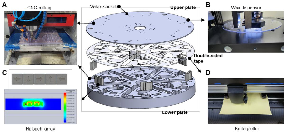
**Figure S4. CTCD fabrication process.** (A) The upper and lower plates of CTCD were machined from polycarbonate slabs by a CNC milling machine. (B) The upper plate has valve sockets to contain ferrowax, which is injected with a precise volume-controlled wax dispenser. (C) Halbach arrays to maximize magnetic force are inserted into the lower plate. (D) The upper and lower plates are assembled by double-sided tape patterned by a knife plotter.
