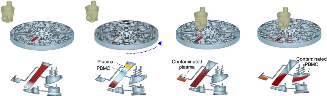
**Figure S1. Conventional laser irradiated centrifugal microfluidic system.** After separating the blood layer, the disc must be stopped for the laser to operate, resulting in spreading the fluid layers. This collapse of the separation results in the imprecise extraction of fluids through the microfluidic channels.
