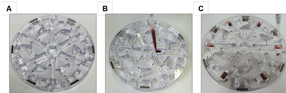
**Figure S6. Blood injection and CTC collection.** (A) An image of the CTCD. (B) Injection of whole blood into the BLOOD chamber via the inlet port of the CTCD. (C) Collection of the CTCs from the CTC chamber via micropipette.
