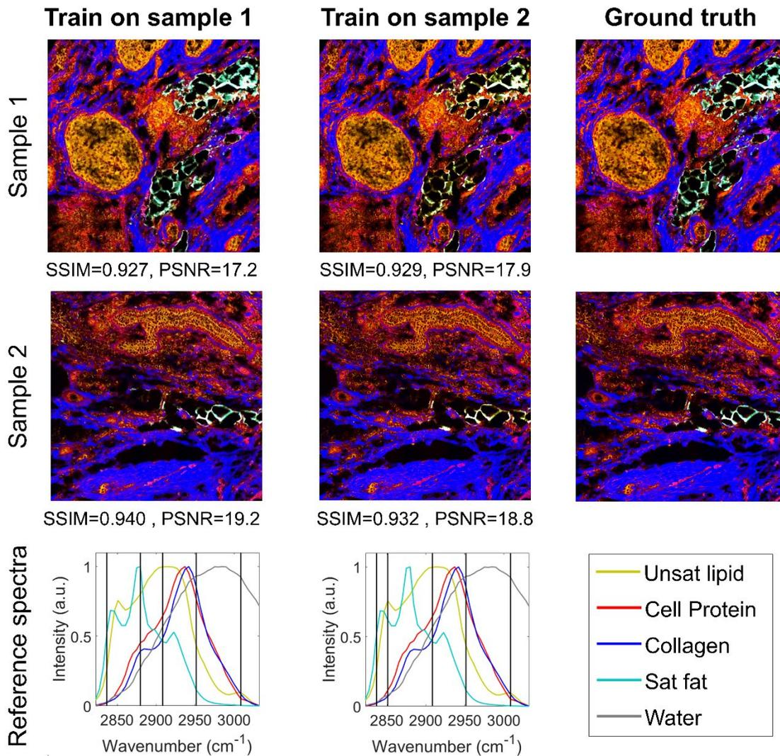
**Figure S1. Comparison of HC-SRH result with different RFE selections.** FOV: 624X627  $\mu\text{m}$ . SSIM: structural similarity. PSNR: peak signal-to-noise ratio.
