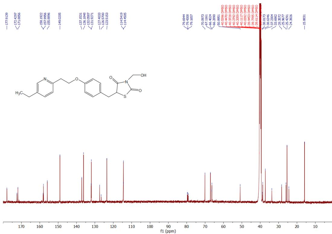
Figure S32: <sup>13</sup>C NMR of compound 20 in DMSO-d<sub>6</sub> (125 MHz).
