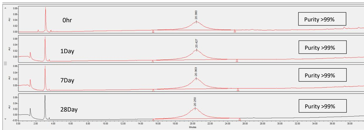
**Figure S39:** Formulation of 2DG-D-Pio in PBS was found to be stable at RT until 28 Days as shown by the HPLC chromatogram @269nm at various time points.
