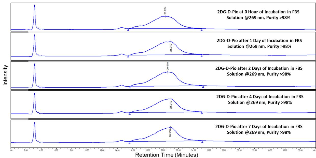
**Figure S41:** *2DG-D-Pio* in 2% FBS in PBS was found to be stable at physiological temperature until 7 Days as shown by the HPLC chromatogram @269nm at various time points.
