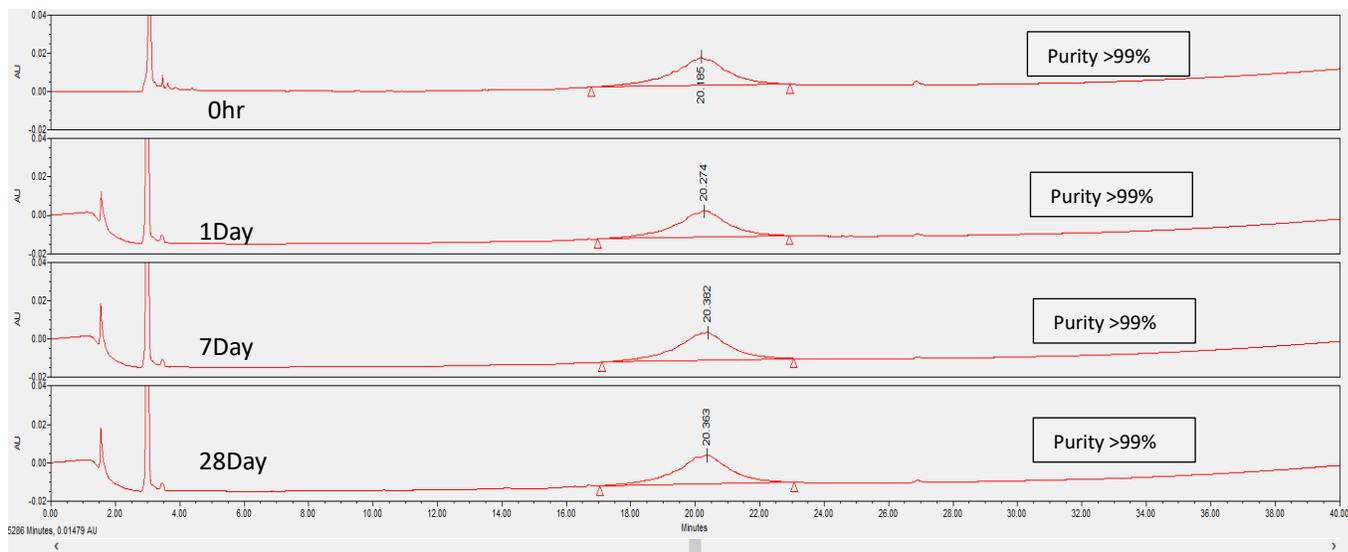
**Figure S40:** Formulation of 2DG-D-Pio in PBS was found to be stable at 4°C until 28 Days as shown by the HPLC chromatogram @269nm at various time points.
