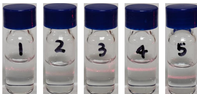
Figure S9. The Tyndall effect of MOC-Mn (dissolved in DMSO) in PBS. The final concentrations are 25, 50, 75, 100, and 125 \mu\text{g/ml} (designated as 1-5 in the picture).
