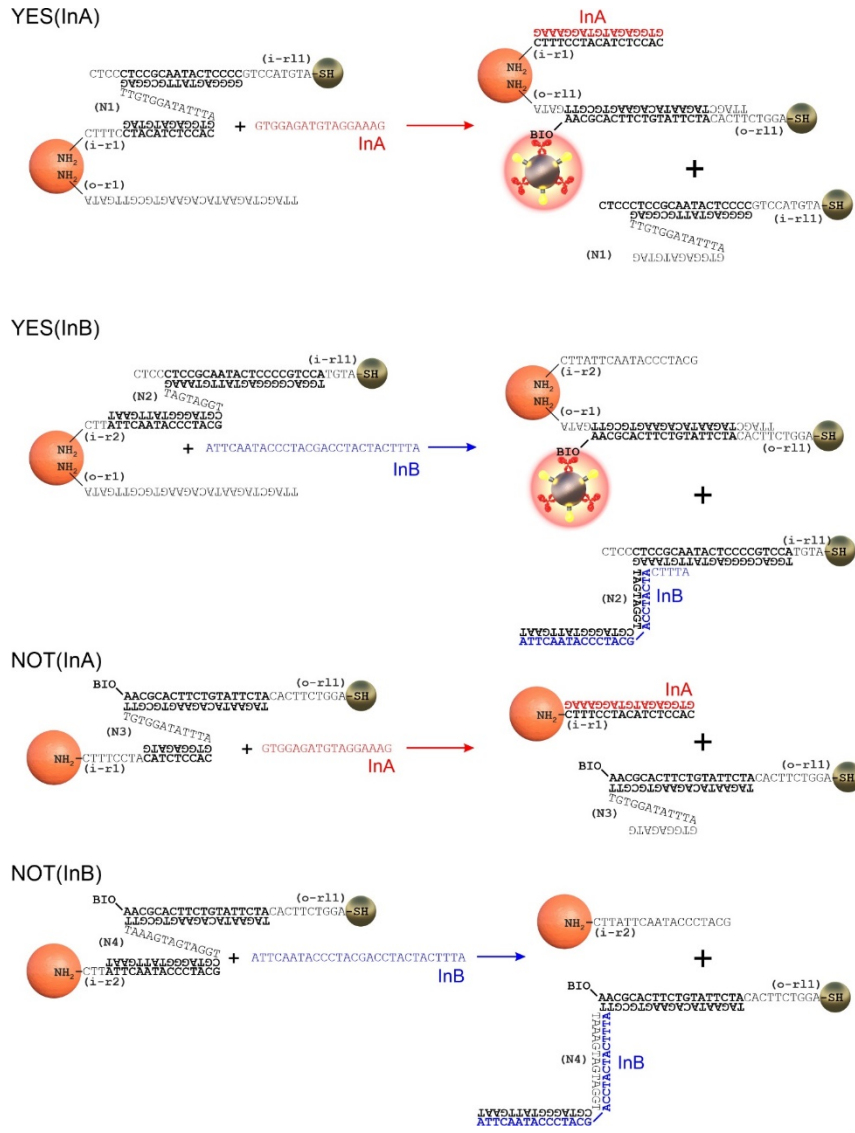
Figure S8. Implementation schemes for YES and NOT gates (see Figure 6 for details).
