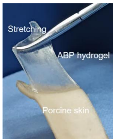
Figure S7 Photographs showing the adhesion behavior of the bottom surface to wet porcine skin surface. The bottom adhesive layer of the ABP tough-bonded to porcine skin.
