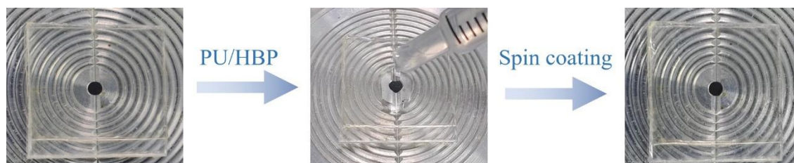
Figure S5 Process diagram of customized Janus for spin coating of the ABP hydrogel.
